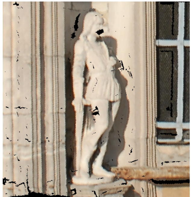
Figure 11. Some example of point clouds created with PhotoModeler 6 Scanner. Point spacing varies from 5 to 10 mm.
