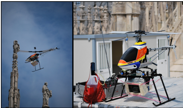
Figure 3. The current RC-Helicopter based on a RC model Hirobo “sst-eagle Freya”, which has been adopted for the photogrammetric surveying of the Dome spire.
