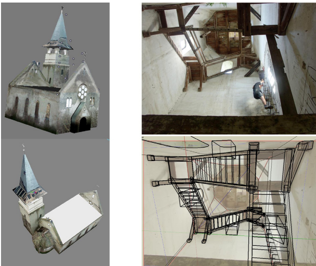
Figure 11. Banostor church. Photogrammetric model on the left and software restitution of interior tower photo on the right
