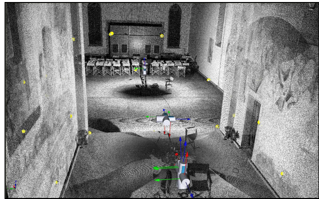
Figure 7. Inner TLS positions and laser points (by intensity).
