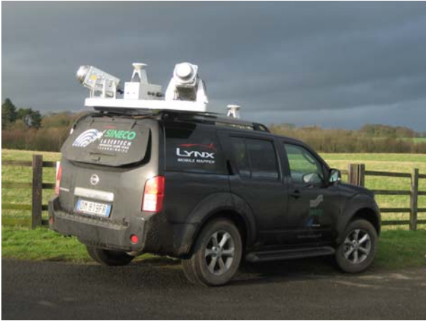
Figure 2: Lynx Mobile Mapper with all the system components
