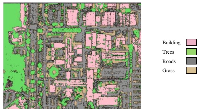
Figure 7: Results of Object-Based Classification
