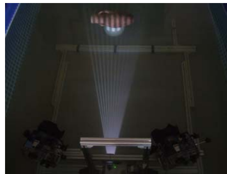
Figure 5. Projection of a pattern during active acquisition.
