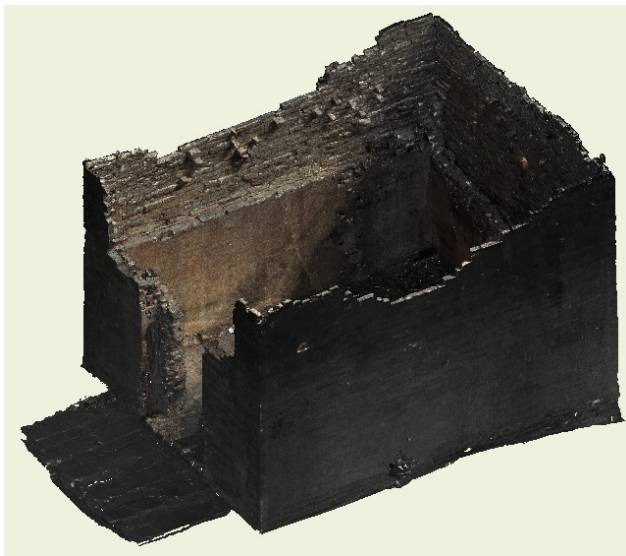
Figure 5: Perspective view of the virtual 3D model of the Almaqah temple, generated as a mesh in the software Geomagic
