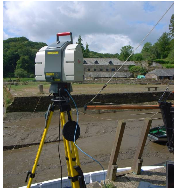
Figure 1 Leica HDS 3000 set-up
