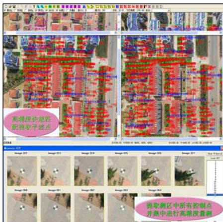
Figure 4 Automatic Aerial Triangulation
