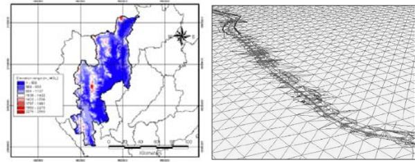
Figure 4. TIN generated from spot heights
