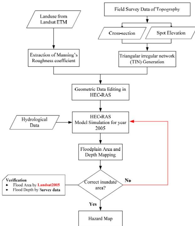
Figure 3. 1D floodplain analysis using HEC-RAS
