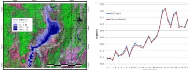
Figure 7. Flood depth verification points (left) Comparison of HEC depth with surveyed depth (right)
