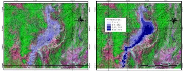
Figure 6. Landsat image (left) compared with flood extent from HEC-RAS (right)
