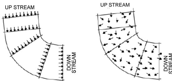
Figure 1. 1D (left) and 2D (right) representations of open channel flow
