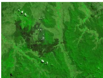
Figure. 3. Multi-spectral (B01, B02, B03, B04-band) fusion map of eastern region of the fire areas
