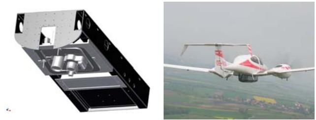
Figure 4. Integration of ADAM into the pod of a DA42 MPP (left: design; right: in flight operation).
