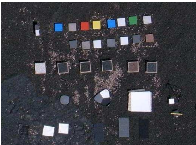
Figure 1. Various reflectance targets at Sjökkulla test field on summer 2009.
