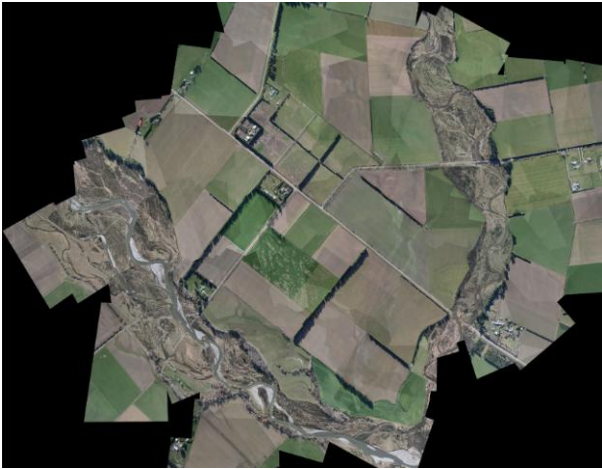
Figure 6. Ortho-image generated from using only in-flight control in the AT (AT Trial 1)
