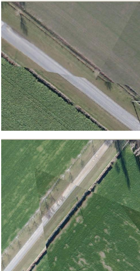
Figure 7. Typical examples of the ortho-image cut lines (AT trial 1)
