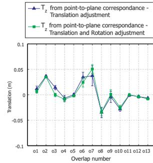
Figure 6: Comparison of vertical offset  $T_z$  estimated by the two adjustment models. The standard deviation bars are scaled up by a factor of 10.
