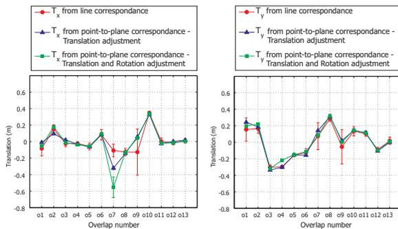
Figure 5: Comparison of 2D translation parameters estimated from line correspondences and point-to-plane distances.
