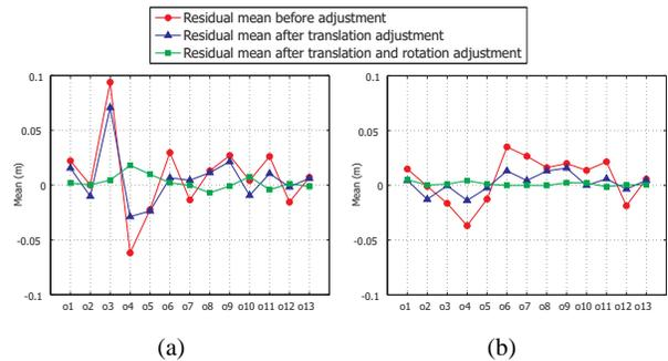
Figure 3: Mean of the point-to-plane distances for 13 overlaps (a) without RANSAC outlier detection, (b) with RANSAC outlier detection.
