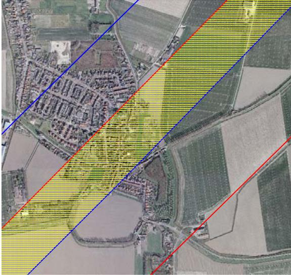
Figure 1: Overlapping strips. The overlap area between the blue strip and the red strip is represented as the yellow hatched area.
