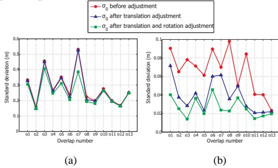
Figure 4: Standard deviation of the point-to-plane distances for 13 overlaps (a) without RANSAC outlier detection, (b) with RANSAC outlier detection.
