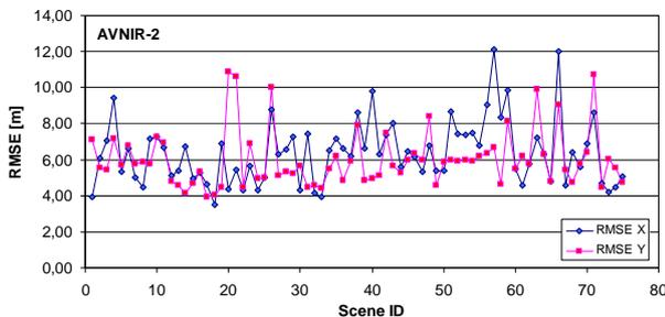
**Figure 4 Geometric accuracy (RMSE) of ALOS AVNIR-2 orthorectified scenes w.r.t. reference images (relative accuracy). RMSE<sub>x</sub> (blue) and RMSE<sub>y</sub> (red)**
