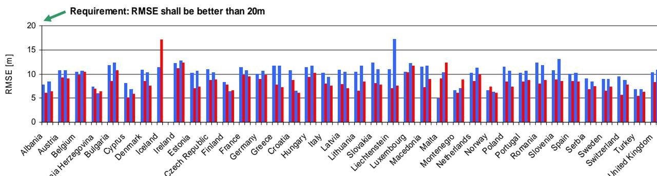
**Figure 3 Geometric accuracy (RMSE) of Image2006 products w.r.t. reference images (relative accuracy). RMSE<sub>x</sub> (blue) and RMSE<sub>y</sub> (red) for European coverage 1 (first two columns of country) and European coverage 2 (last two columns of country)**
