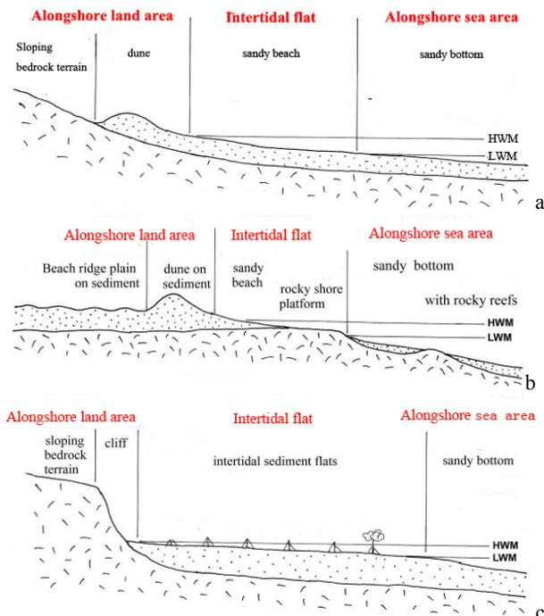
Figure3 Profile sketch map of three coastal type of bays.(a) sandy coast; (b) rocky coast; (c) silty coast.HWM stands for meanHigh-water Mark, LWM stands for mean Low-water Mark
