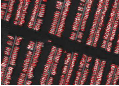
Figure 9: Extraction results favoring aligned ellipses having a particular direction: 523 ellipses ( \beta = 1000 , \gamma_d = 27.56 , \gamma_{al} = 9.18 , s = 0.3 , d_0 = 6 ).
