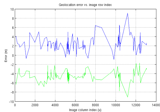
Figure 3. The effect of image row in UTM Y (blue) and UTM X (green) errors.
