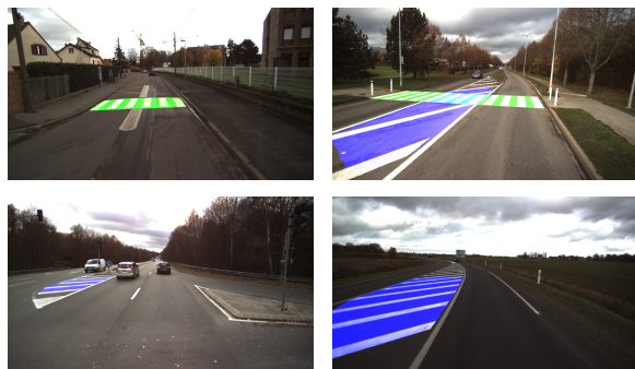
Figure 12: Example of experimental images with algorithm result. Blue areas represent hatching lines detection and green one represent zebra-crossing detection.
