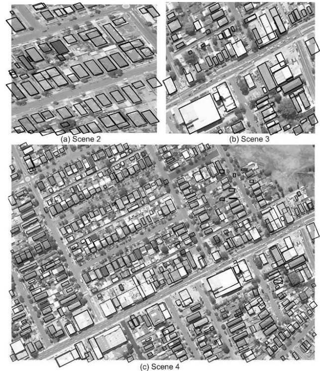
Figure 6: Detected buildings on the orthoimages.
