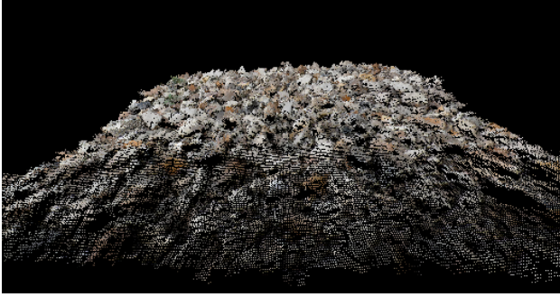
Figure 14: 3D view of the pebble with total surface roughness Sq=0.1668029cm, Sa=0.122973cm and SD=0.112528cm
