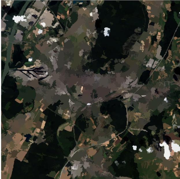
Figure 10: Landsat Scene after segmentation (Channels: R=3, G=2, B=1)
