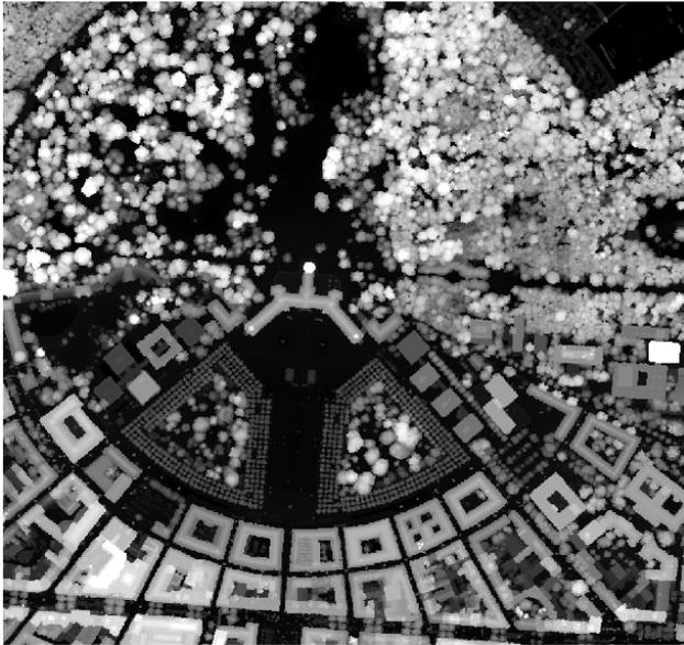
Figure 6: LiDAR Scene (Shown : First-Pulse)
