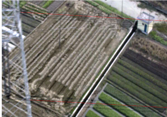
(b) power line extraction result Figure 5. experiment with real data
