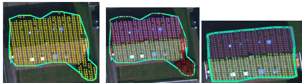
Figure 13. Left:detected building outline(cyan) and LIDAR points(yellow), Middle:detected roof plane points(purple-green) and non-roof points (red), Right:New building outline after elimination of non- roof points
