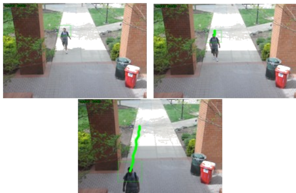
Figure 6. Object detection and tracking. The green rectangles show the detection results (upper body detection), and the green curve shows the trajectory of the person.
