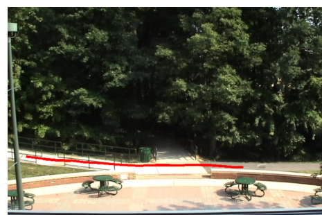
Figure 5. The trajectory of the moving person detected in the video feed of Fig. 4, overlaid on the background frame.
