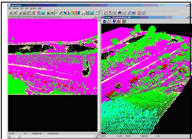
Figure 5. Full Classification of LiDAR Points
