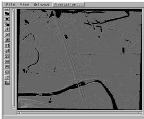
Figure 1c. DTM Voids Filled With Inpainting
