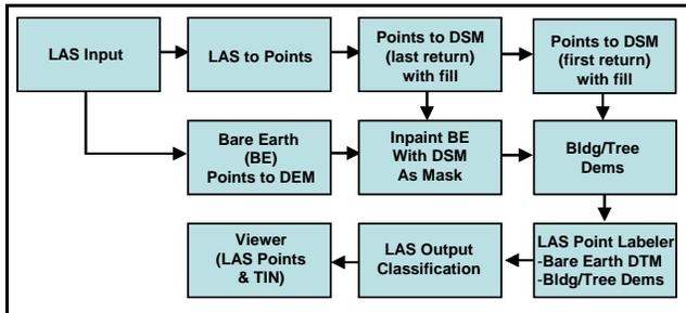
Figure 2. LiteSite® LiDAR Classification Processing Flow Diagram
