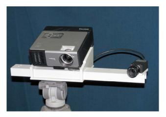
Figure 1. The projector-camera photogrammetric system
