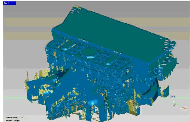
Figure 9. 3D model triangulated in Geomagic software.
