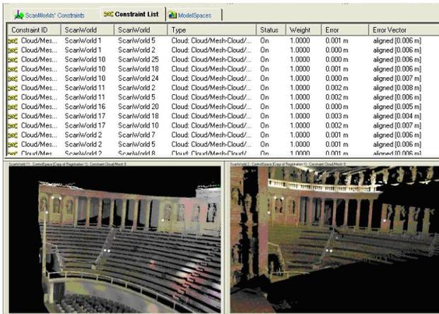
Figure 7. Pairwise scan alignment.
