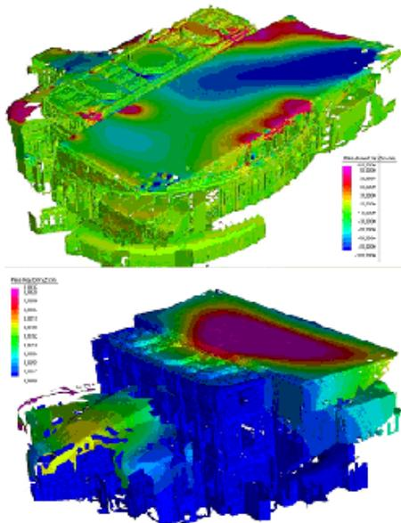
Figure 11. Results of the *Static Analysis* applied to the laser scanner 3D model of the *Olympic Theatre*.
