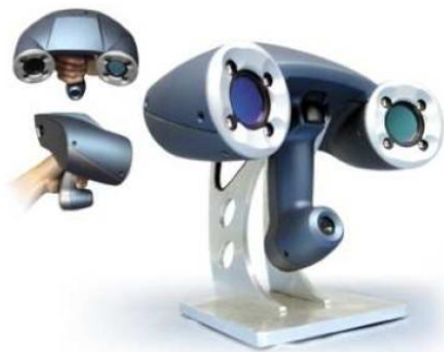
Figure 2. Handyscan 3D: the acquisition unit (980 g, 160 x 260 x 210 mm)
