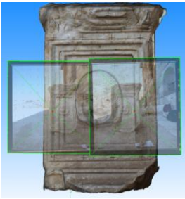
Figure 16. The photogrammetric position of two images employed for the texture phase
