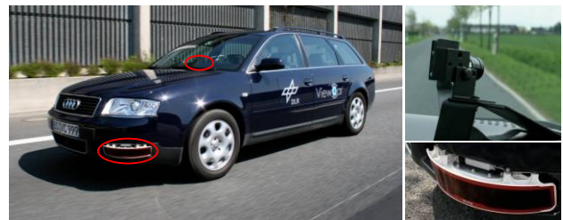
Figure 1. Experimental platform, the ViewCar, containing a laser scanner and a camera (among other sensors).
