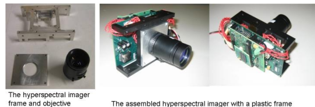
Figure 3: The parts of Staring FPI Hyperspectral Imager and an integrated equipment. The envelope is 100 mm x 70 mm x 53 mm, The objective tube extends out of the main structure by 35 mm.
