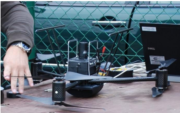
Figure 4: VTT Staring FPI Hyperspectral Imager integrated on VITO six-rotor rotorcraft type Draganfly X6
