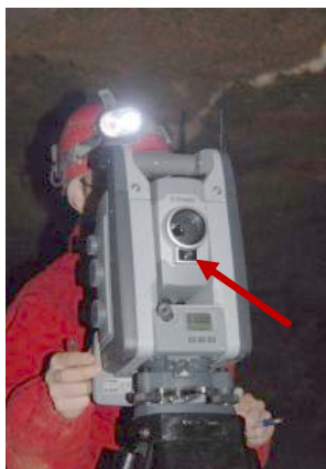
Figure 7: The Trimble VX TM spatial station is equipped with a 3 Megapixel built-in camera (just below the telescope of the instrument)
