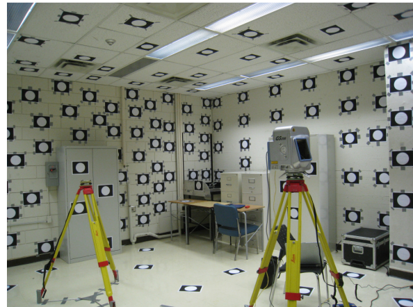
Figure 1: Instrument setup during the first calibration
