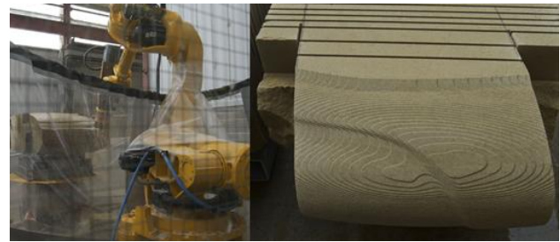
Figure 9. 6-Axis robotic machining (left) and an example of the textures applied to the planters during machining (right).
