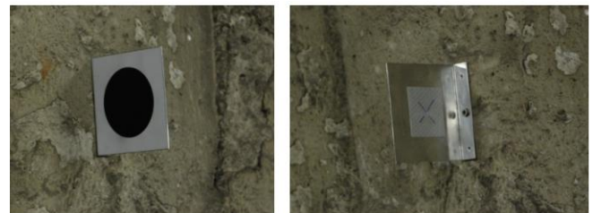
Figure 2. The “double face” target for photogrammetric and theodolite measurements.
