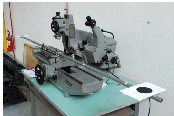
Figure 8. For narrow tunnels a 3-4 m calibrated bar (e.g. a telescopic tube) can substitute the wire and remove the scale ambiguity of the photogrammetric project.
