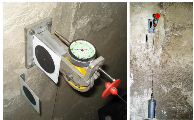
Figure 3. The wire and the gauge used to remove the scale ambiguity from the photogrammetric project.
