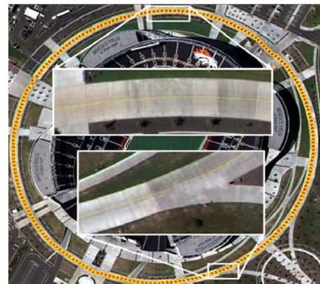
Figure 5. The extracted ring road of a stadium by our proposed method (Note that the rectangular template matching method failed on this image)
