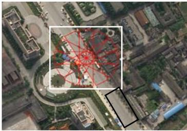
(a) A rotating rectangular template and its resulted sub-windows
