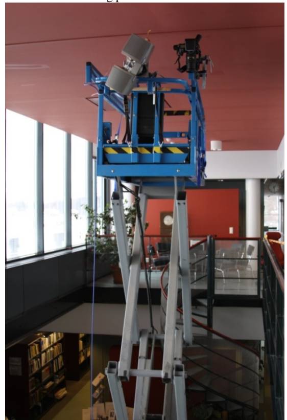
Figure 2. The FARO scanner at the 9 m high position. Photo J. Hyyppä.
