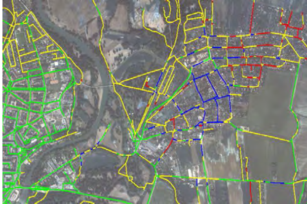
Figure 9: Detail of result of damage assessment system using all available input data: image t_1 , image t_2 , DEM and manual generated reference at time t_1 . (green = trafficable , yellow = possibly flooded , red = flooded , dark blue = flooded \Rightarrow trafficable ).
