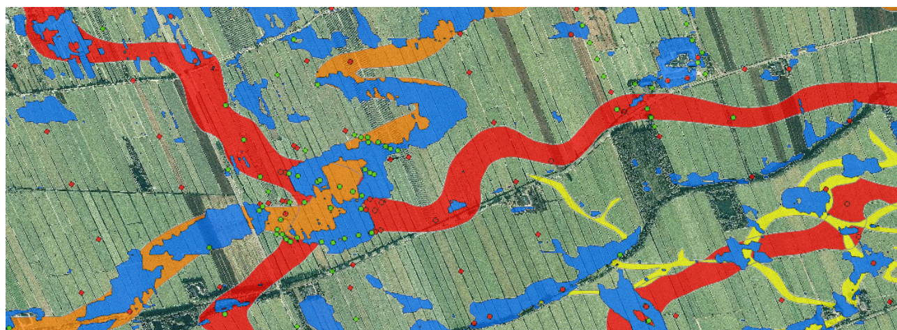
Figure 8: Buried channel classification results. Blue: Automatic classification LIDAR data; Red, orange, yellow: classification according to digital paleogeographic map, compare Fig. 1; Red dots: DINO drillings classified as non-channel; Green dots: DINO drillings classified as channels.
