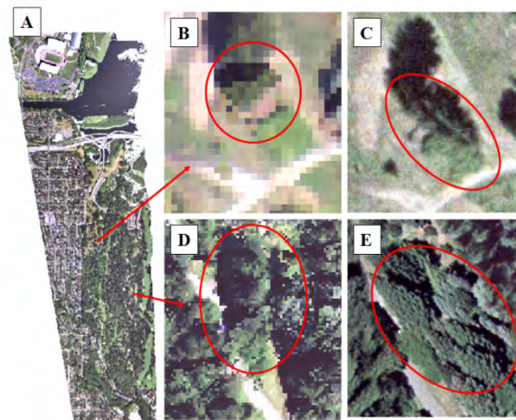
Figure 3. The true orthophoto generation. The final product of true orthophoto for the entire area (A). Single tree shown on the trueortho (B) and the same tree shown on USGS orthophoto (C). A group of trees shown on the trueortho (D) and the same trees shown on USGS orthophoto (E).
