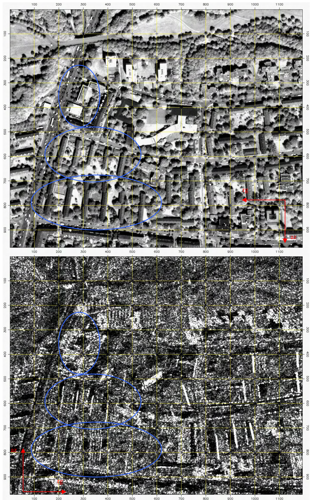
Figure 8. Part of Munich city acquired by IKONOS (upper image) and TS-X (lower image) using the accidental satellite formation. Yellow grid lines are for better orientation between two images. Red arrows show flight (az) and look (rg) directions.
