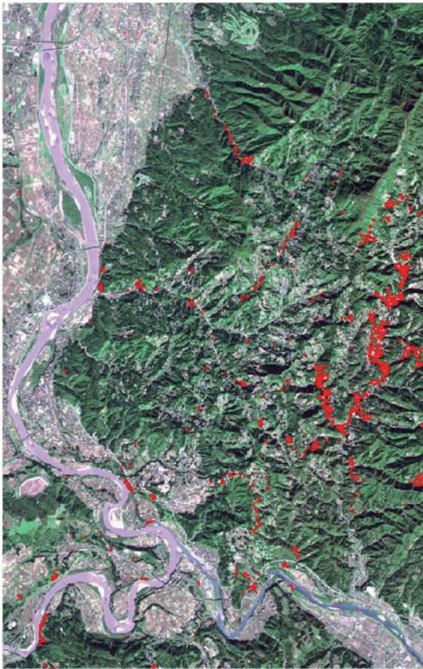
Figure.6 Detected damage area by *NDVI* analysis
