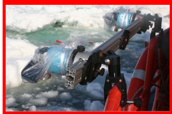
(b) Two HDV cameras attached on the back side guardrail of the icebreaker.
