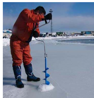
(a) Drill a hole on the sea ice
