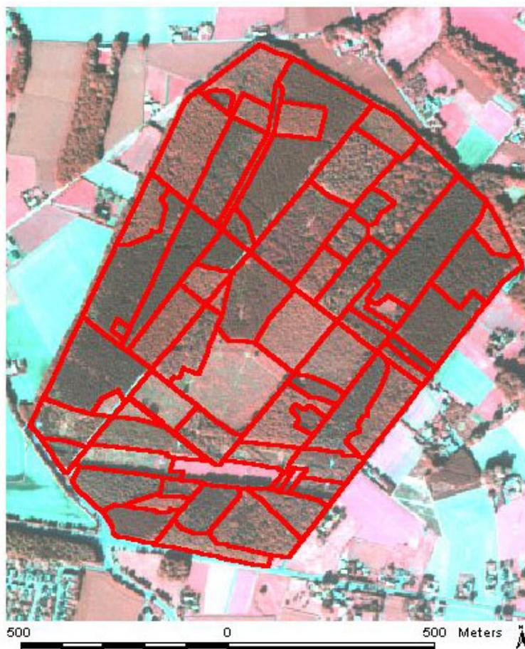
Figure 2. Registering of the stand borders based on aerial CIR photos
