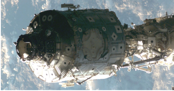
Figure 12. The existing Space Vision System uses the known locations of the B/W targets to compute the pose of objects (Photo reproduced with permission from NASA).
