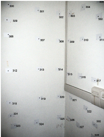
Figure 3 Calibration targets placed on walls.
