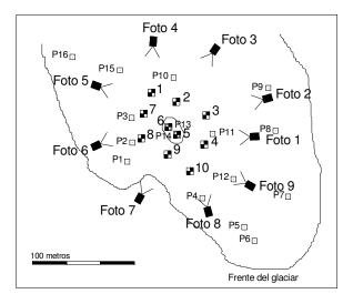
Figure 4. Scheme of the rods, control points or artificial signs of the photographics takings.
