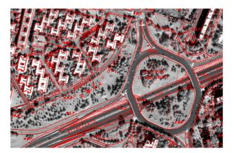
Figure 9. Overlay of portion of the raster orthoimage and the map layer. Comparison of the main features highlights differences between products
