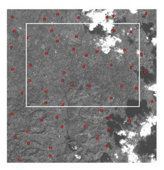
Figure 3. QuickBird image illustrating the point dataset acquired with the DGPS survey and, in the white rectangle, the EROS image limits
