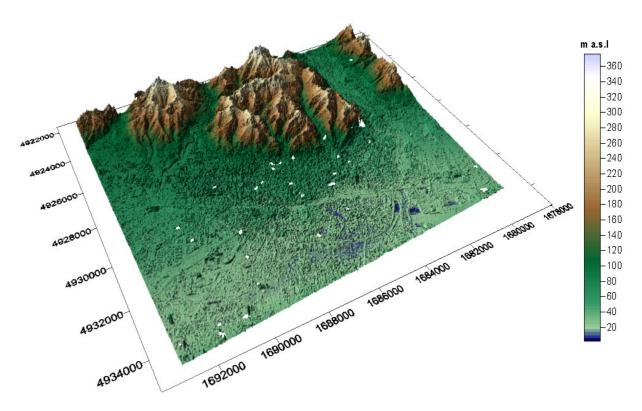
Figure 5. Geocoded Digital Surface Model. Elevation. Coordinates are expressed in the National - Gauss-Boaga grid. Holes, depending on the failure of the correlation phase, are visible in figure as white area.
