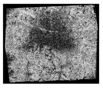
Figure 4. Correlation index plotted as grey levels; white pixels indicate the full correlation whereas black pixels indicate a low correlation or correlation failure
