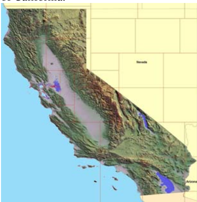
Figure 3: NEXTMAP USA Example - California DSM Validated vertical accuracy (1430 check points) 0.76 m RMSE
