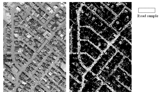
Figure.3 Result of image segmentation Left: input image Right: road seed
