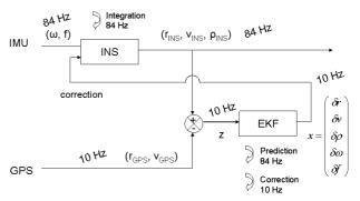
Figure 4: GPS-INS coupling
