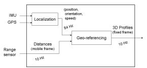
Figure 2: framework for construction of 3D points
