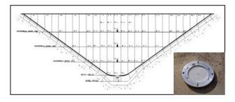
Fig. 2.- Positions of targets to be used as independent control points on the dam's front; in the window on the left, an image of a retro-reflecting target used for Riegl LMS-Z420i laser scanner.
