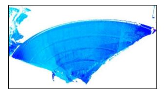
Fig. 4.- Point-cloud resulting from data fusion of all scans capturing dam downstream face acquired by Leica HDS 3000.
