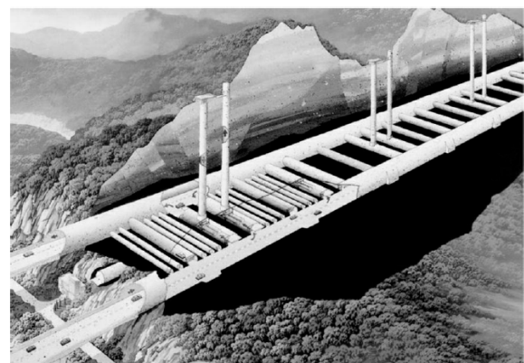
Figure 2. Ventilation System of Hsueh-Shan Tunnel
